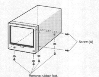
When mounting the monitor on the rack mount chassis, fix the monitor to the blank panel with M3x8 screws. Use four M3x8 screws to fix the monitor on the chassis.
