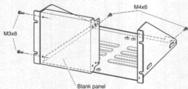
Illustrations as shown below are examples mounting the monitor on the left side.
